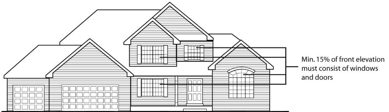
Figure 3: Calculating Area of Façade Devoted to Windows and Doors
